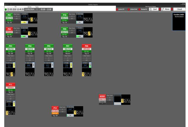
Our synoptic is equal to the **corporate layout** of production departments. We have **real-time useful information**, such as machine status, duty cycle, order progress, various alarms set up from personal data, the operator code, etcetera. **Connection to machines** is defined according to the type of machine itself.
