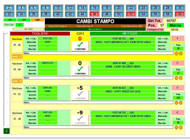
**Scheduling** is carried out from the office desk to machine ui. **A simple and intuitive interface** shows the sequence of mold changes to be made on every machine.
