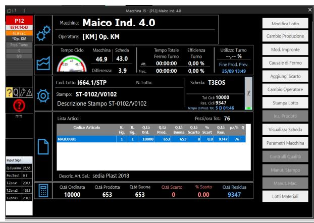
**Department Operator**, using machine synoptic, can display information on **production**, such as duty cycle progress, rate of job progress, downtime during shift, expected end time and so on.
